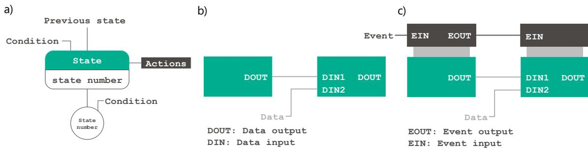
**Fig. 2: Qualitative representations of the three standards commonly used in the automation industry: a) State machine (VDI 3812-14); b) FBD (IEC 61131-3); c) FB (IEC 61499).**
