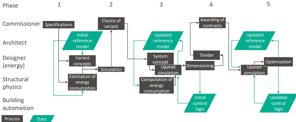
Fig. 3: BIM Use-Case. Simplified schematic representation of Operational Procedure (Meier, 2018).
